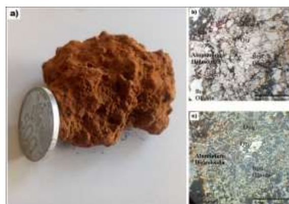
Figure 4. Microdiorite bauxite concretion sample. (a) megascopic scale of bauxite concretion, (b) parallel polarization petrographic of bauxite concretion, (c) cross polarization petrographic of bauxite concretion.
