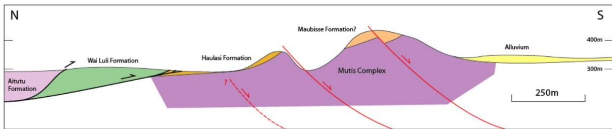
**Figure 6:** Cross-section through the Mutis massif in Noil Meto. No vertical exaggeration. Line of the section is in Figure 5.
