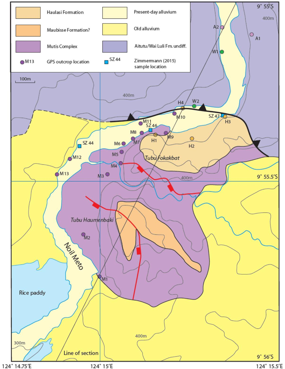
**Figure 5:** Geology of the lower section of Noil Meto from GPS-constrained fieldwork and interpretation of Google Earth imagery. Topography at 50m interval contoured from Google Earth.
